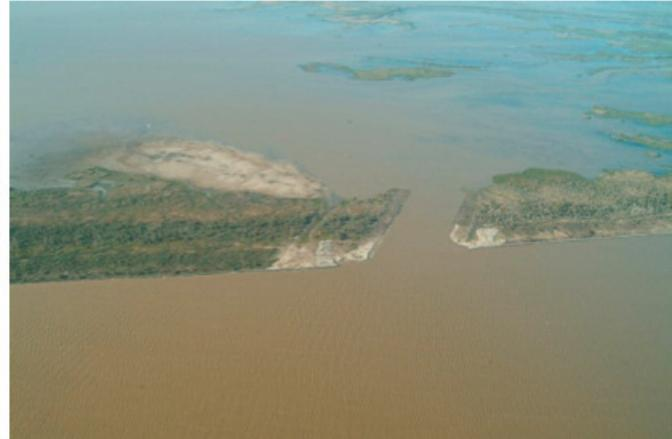
The conveyance channel allows fresh water and sediment to flow from the Mississippi River (bottom of picture) to restore vegetated wetlands in an area that is currently shallow open water.
